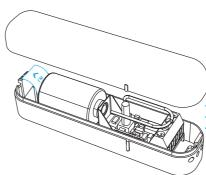
2. Remove the battery blocker.
